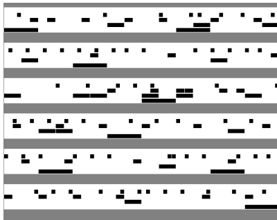
Fig. 7. Interleaving the 120 detail coefficients at levels 4-7 from a Haar wavelet decomposition of a signal of length 128.
